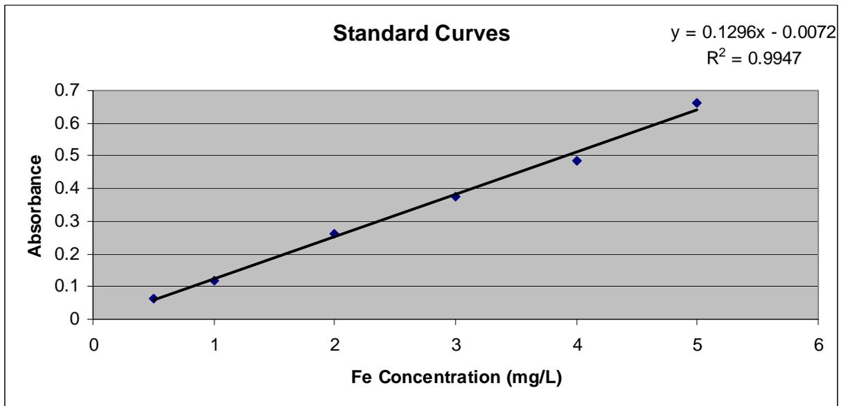
*This is the second standard curve constructed during the titration study.*
