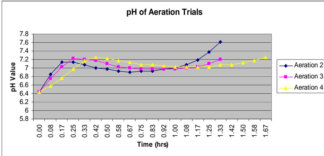
Figure 9 displays the pH value for each trial in relation to the time during aeration.
