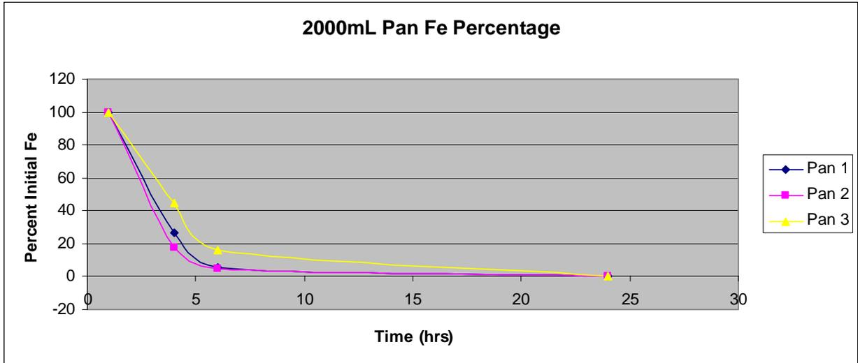
Figure 13 indicates the percentage of iron remaining in solution over time for each trial using a pan with a 2000mL sample volume.
