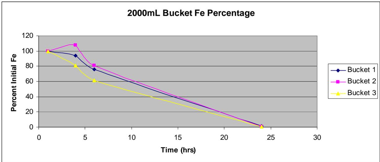
Figure 14 displays the percentage of iron remaining in solution over time for each bucket trial with a 2000mL sample volume.
