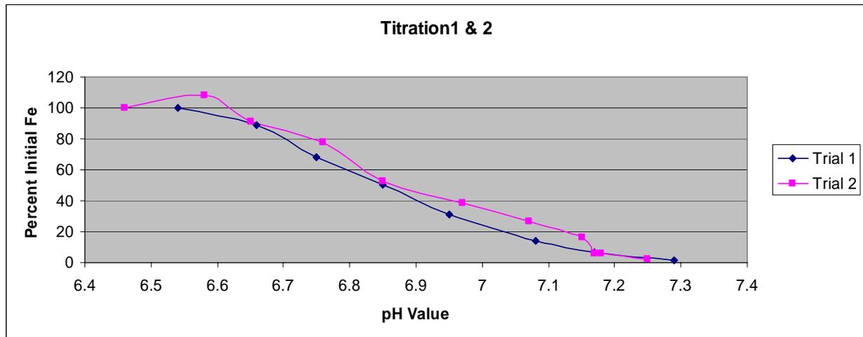
Figure 7 displays the percentage of iron left in sample as compared to the initial concentration in relation to increasing pH.
