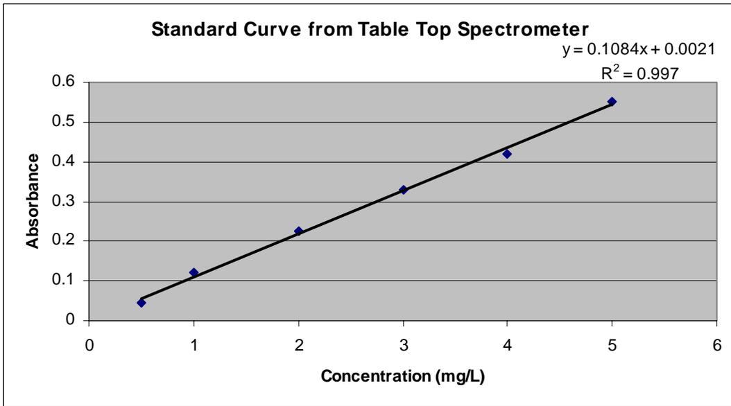
This is the standard curve constructed when having to use the Table Top Spectrophotometer (Spectronic 20 Genesys).
