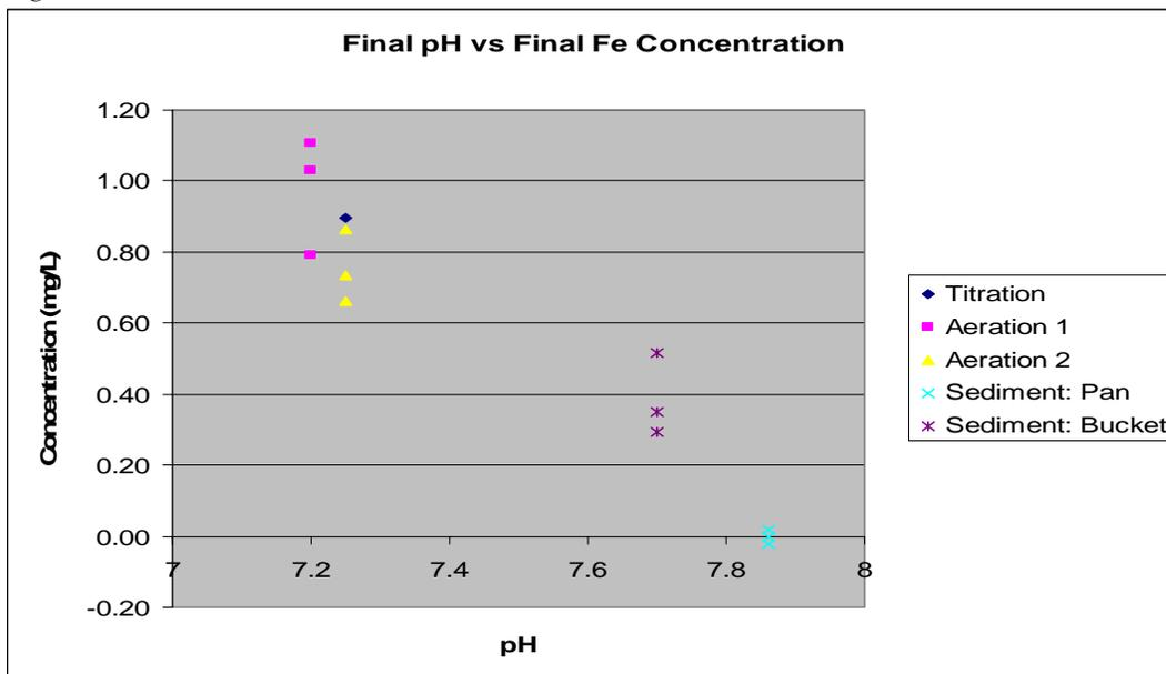
Figure 16 displays the relation between final pH values and final ferrous iron concentrations for each study performed.
