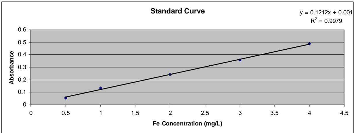
Figure 6 is the standard curve constructed for the pH, aeration and settling pond studies.
