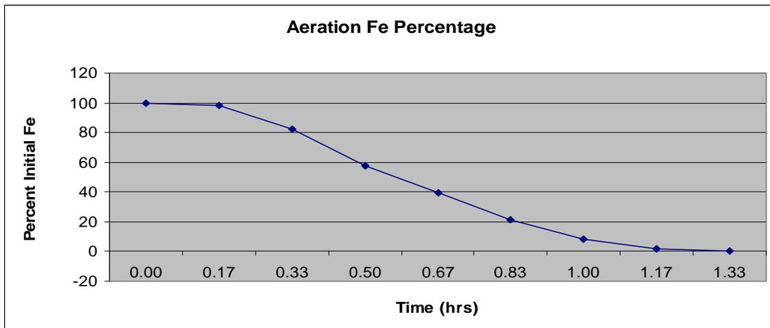
Figure 10 indicates the percent of ferrous iron present as it correlates to the amount of time for it to precipitate out of solution through aeration.
