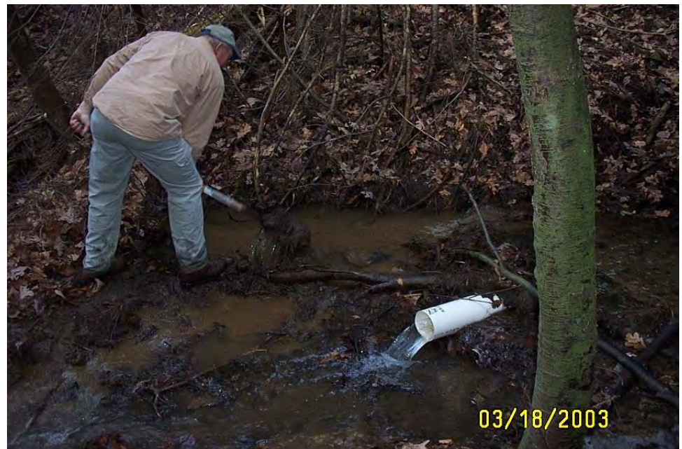
☐ Photo 4: NB12D. The flow rate of the discharge was measured from the pipe as shown.
