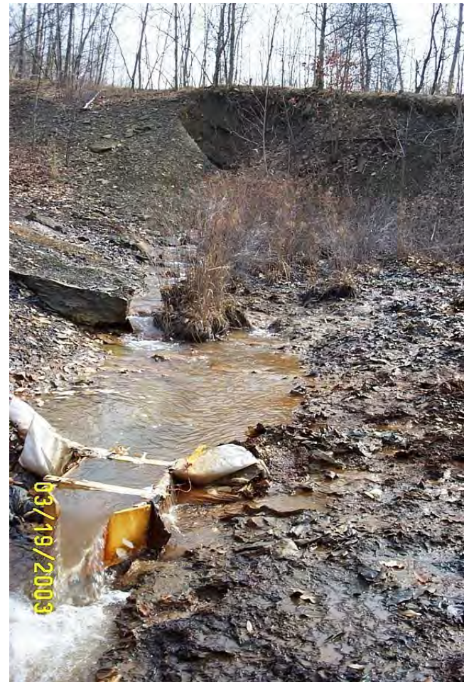
☐ Photo 24: NBG15D. The discharge was sampled at the flume in the lower left of the photograph. The culvert is in the background.
