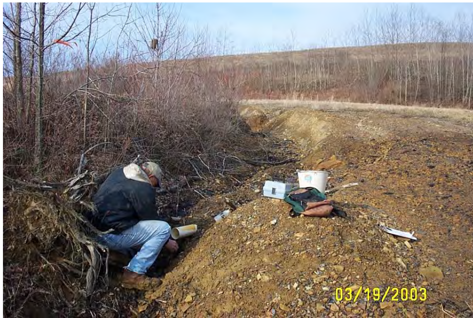
☐ Photo 25: NBG25D. The discharge emerges from reclaimed mine spoil which is shown in the background. The discharge was collected and sampled in this erosion channel.
