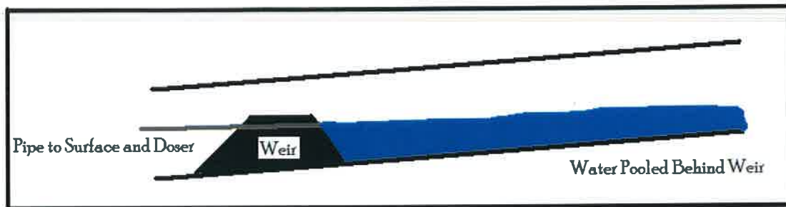
Figure 13. Profile of the technique that will be utilized to capture the “Lucerne 3A” Mine Discharge at the desired surface elevation.
