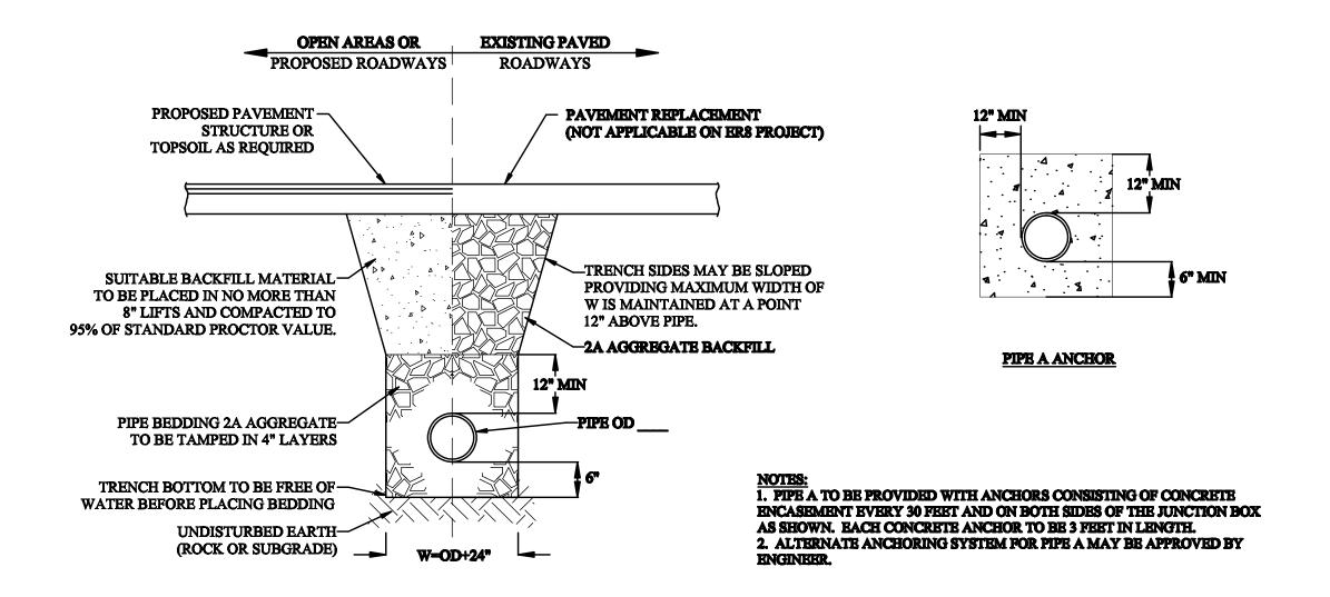
TRENCH AND ANCHOR DETAIL FOR CONVEYANCE PIPING UNDER OPEN AREAS AND ROADWAYS
