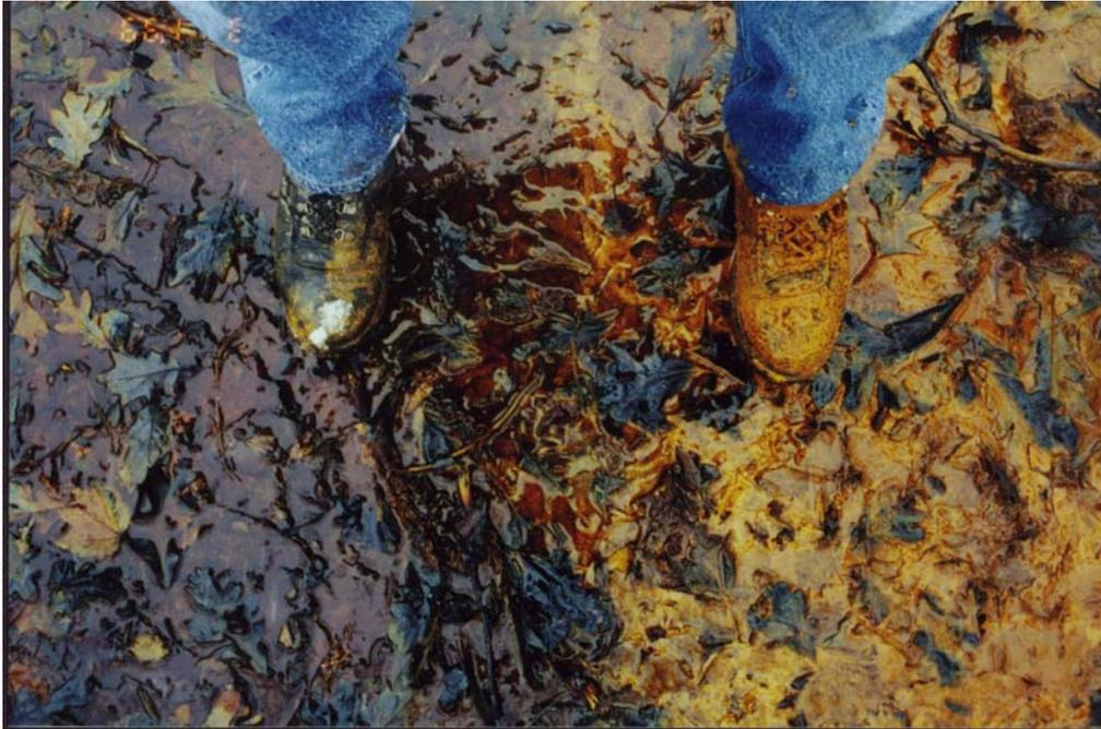
Iron precipitates at discharges 12 and 13 prior to passive treatment system installation. (3/1/99)
