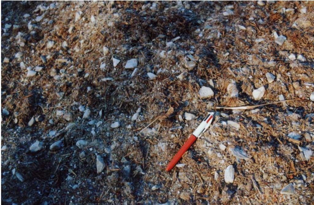
Spent mushroom compost and limestone aggregate mixture overlying 600 tons of limestone in Vertical Flow Pond. (11/19/99)
