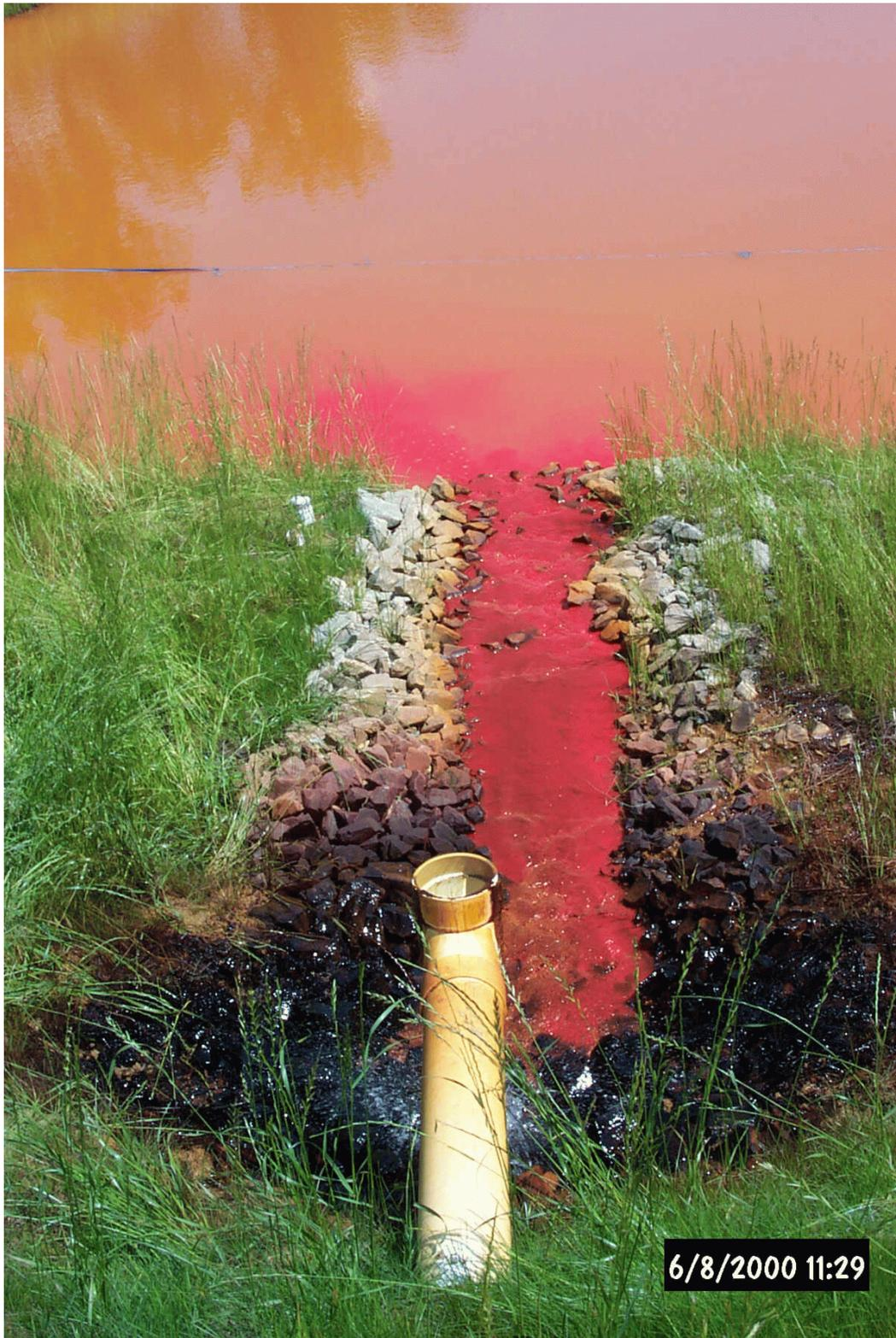
Beginning of dye test of Settling Pond #1 examining water distribution patterns.
