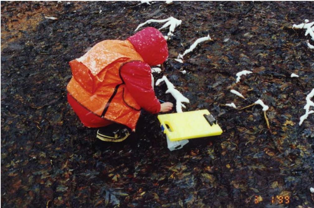
Sampling diffuse flow of discharges 12 and 13 prior to passive treatment system installation. (3/1/99)
