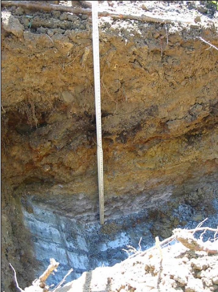
Test pits were dug to determine soil profile and depth to Brookville coalbed and the associated mine pool.
