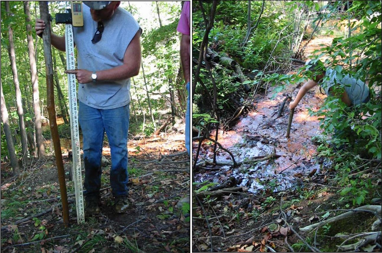
John Stoops, foreman for Quality Aggregates Inc., roughly measures the depth of iron precipitate that has accumulated from the 87-7 discharge. Notice the depth of sludge within the channel was over 42"!!!
