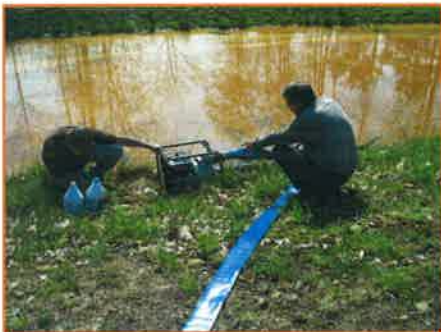
The suction line would effectively remove sludges from a twenty foot radius. The trash pump was capable of removing leaves that had blown into the pond.
