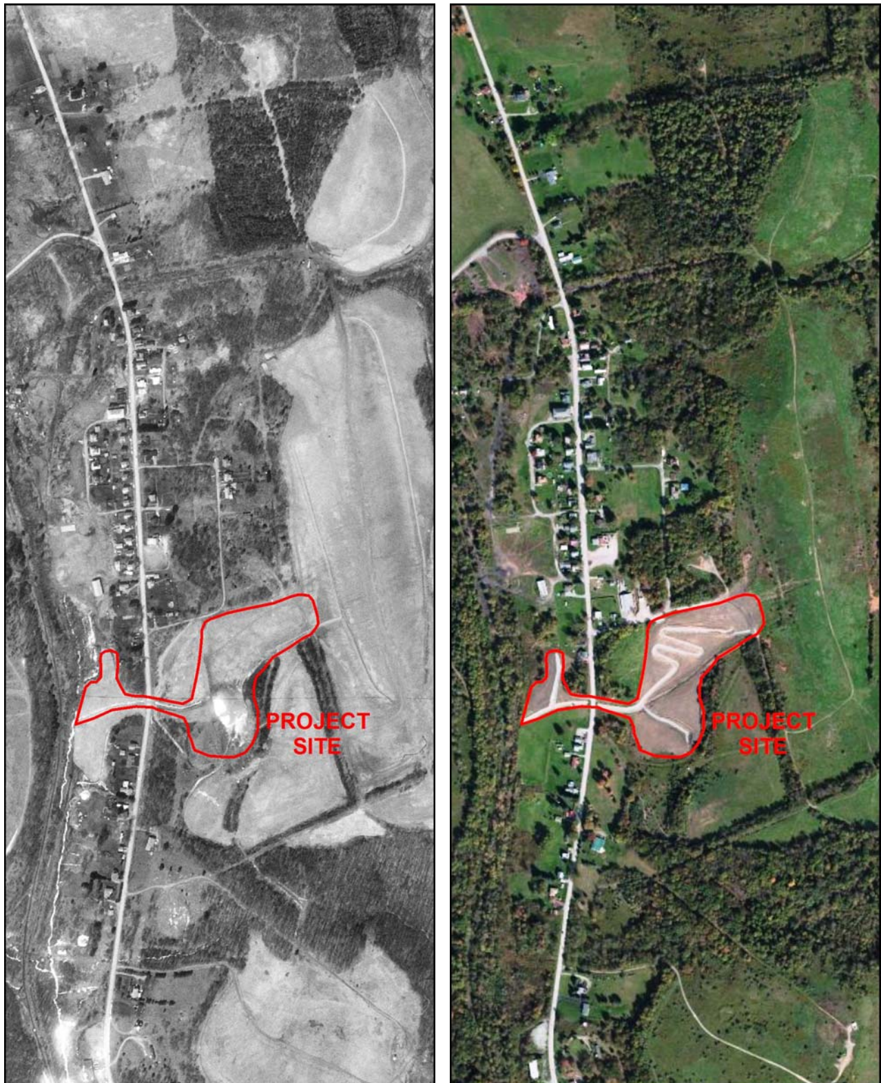
Figure 4: Comparison of aerial photos from 1993 (left) and 2011 (right). The 1993 aerial photo shows the recently reclaimed coal refuse site. Coal refuse was spread further south for stabilization and to attempt to extinguish the fire. The 2011 aerial shows the newly constructed treatment system.
