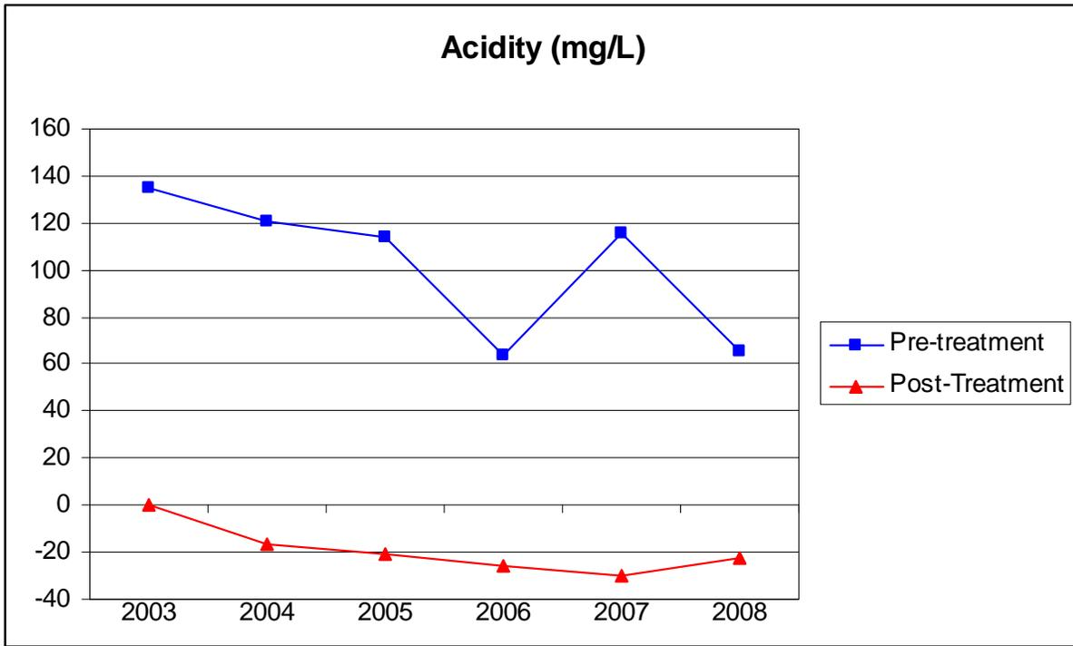
Negative values show that net alkalinity has been added to the final effluent.
