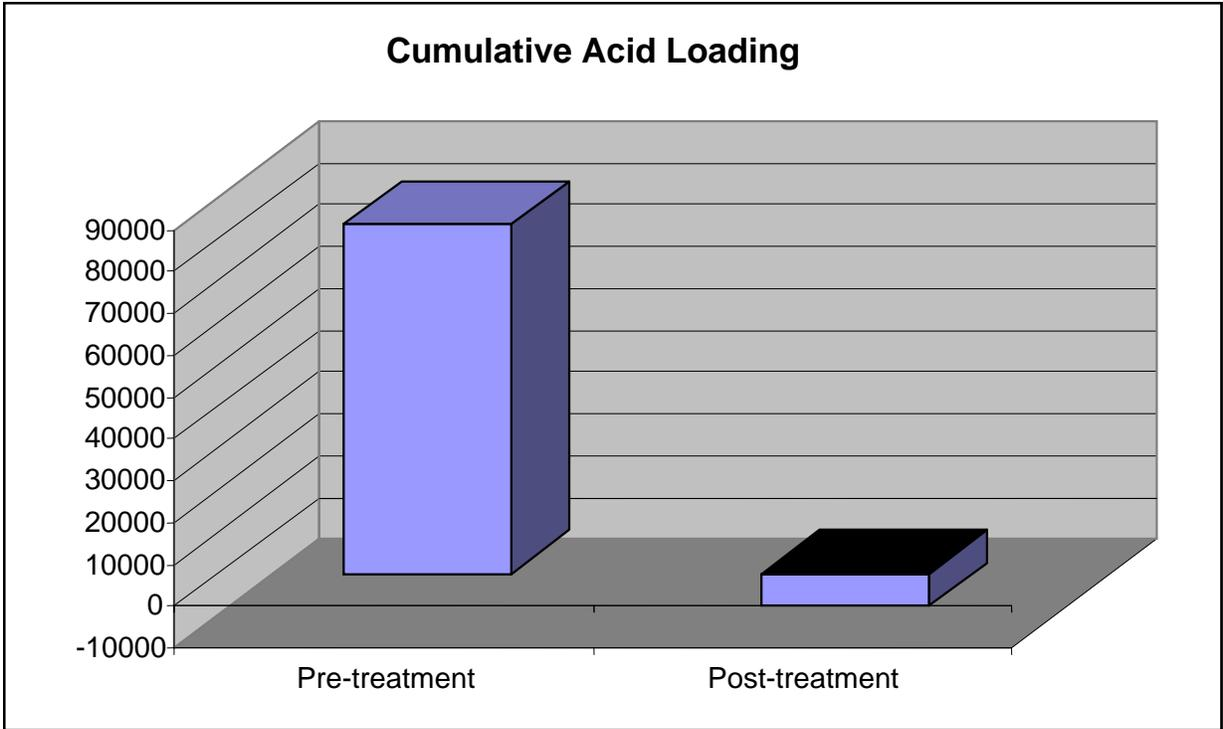
83,470 lbs of acid have been removed and 7,624 lbs of alkalinity have been produced since 2003.
