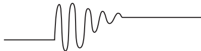
The signal oscillates between states after a mechanical switch or relay activates.
