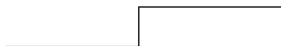
With a debounce filter, the signal is interpreted to change state only once.
