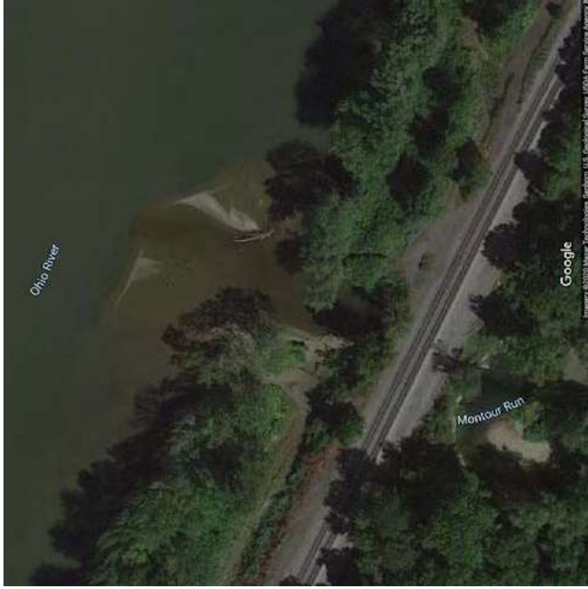
Figure 2.1.2 -Sediment-laden water drains from Montour Run (center, bottom of image) into the Ohio River. Blue arrows indicate two regions of visible sediment accumulation. Image downloaded from Google Maps-Imagery 2020
