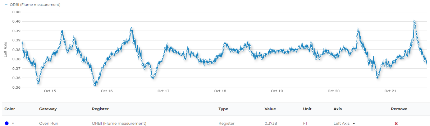
Figure 2. Flow Depth at H-Flume Example
