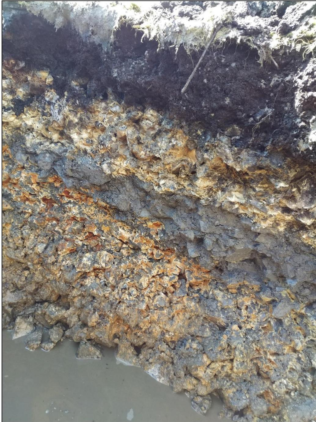
Test pit within Oven Run B SAP1. An algal mat covered the entire pond. Below the algae was often a layer of iron on top of the compost. The limestone was often coated in iron and aluminum precipitates, but there were also “lenses” of clean or mixtures of clay and limestone that did not appear to have contact with AMD.
