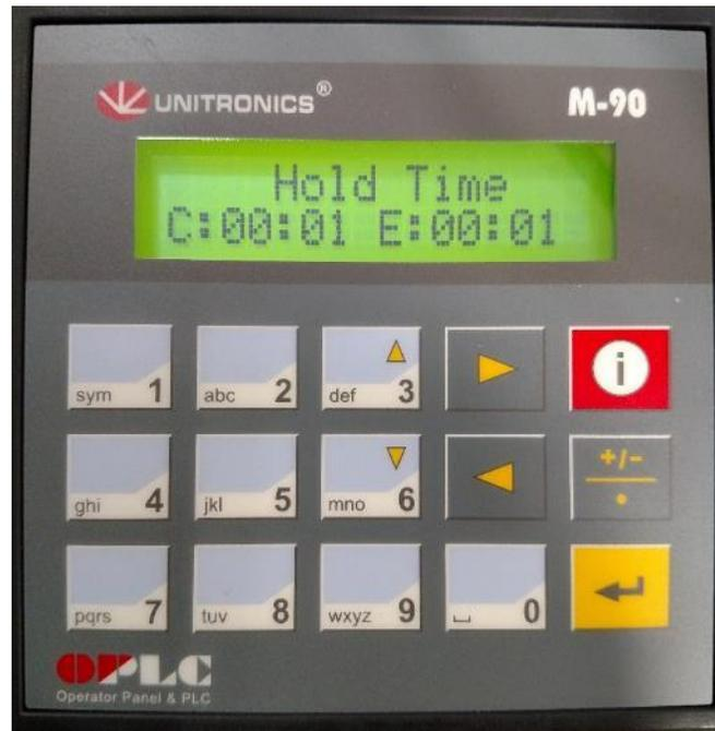
**C:** Displays the current Hold Time setting in hh:mm format (in the picture, the current Hold Time is 1 minute.)
