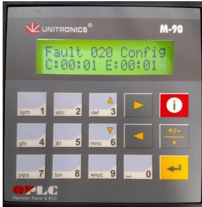
C: Displays the current timeout for fault 020. The default timeout is 00:05 minutes before a fault is indicated on the Faults screen
