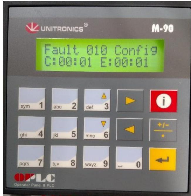
C: Displays the current timeout for fault 010. The default timeout is 24:00 hours before a fault is indicated on the Faults screen
