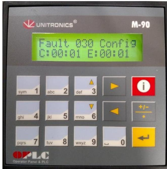
C: Displays the current timeout for fault 030. The default timeout is 24:00 hours before a fault is indicated on the Faults screen
