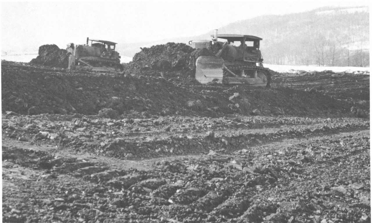
FIGURE 21. - Comparison of the Moving Capacity of Two Types of Blades: Boulderson Blade (Foreground) and U-Blade (Background).
