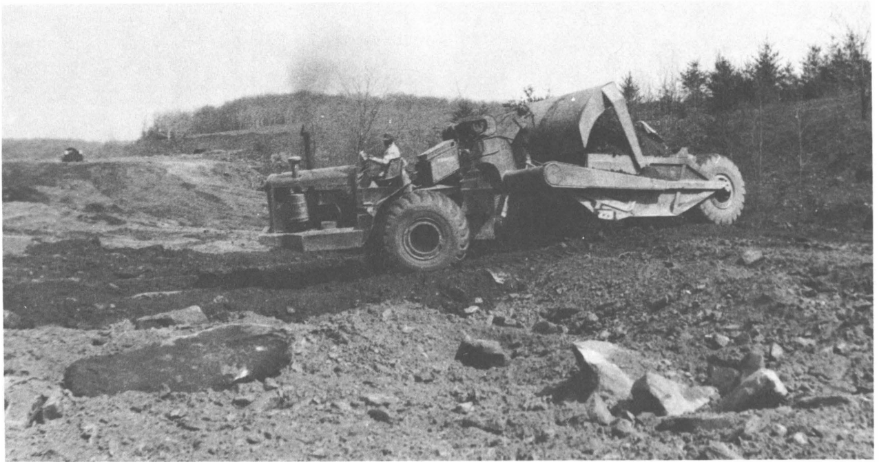
FIGURE 22. - Scrapers Move More Material Per Haul Cycle.
