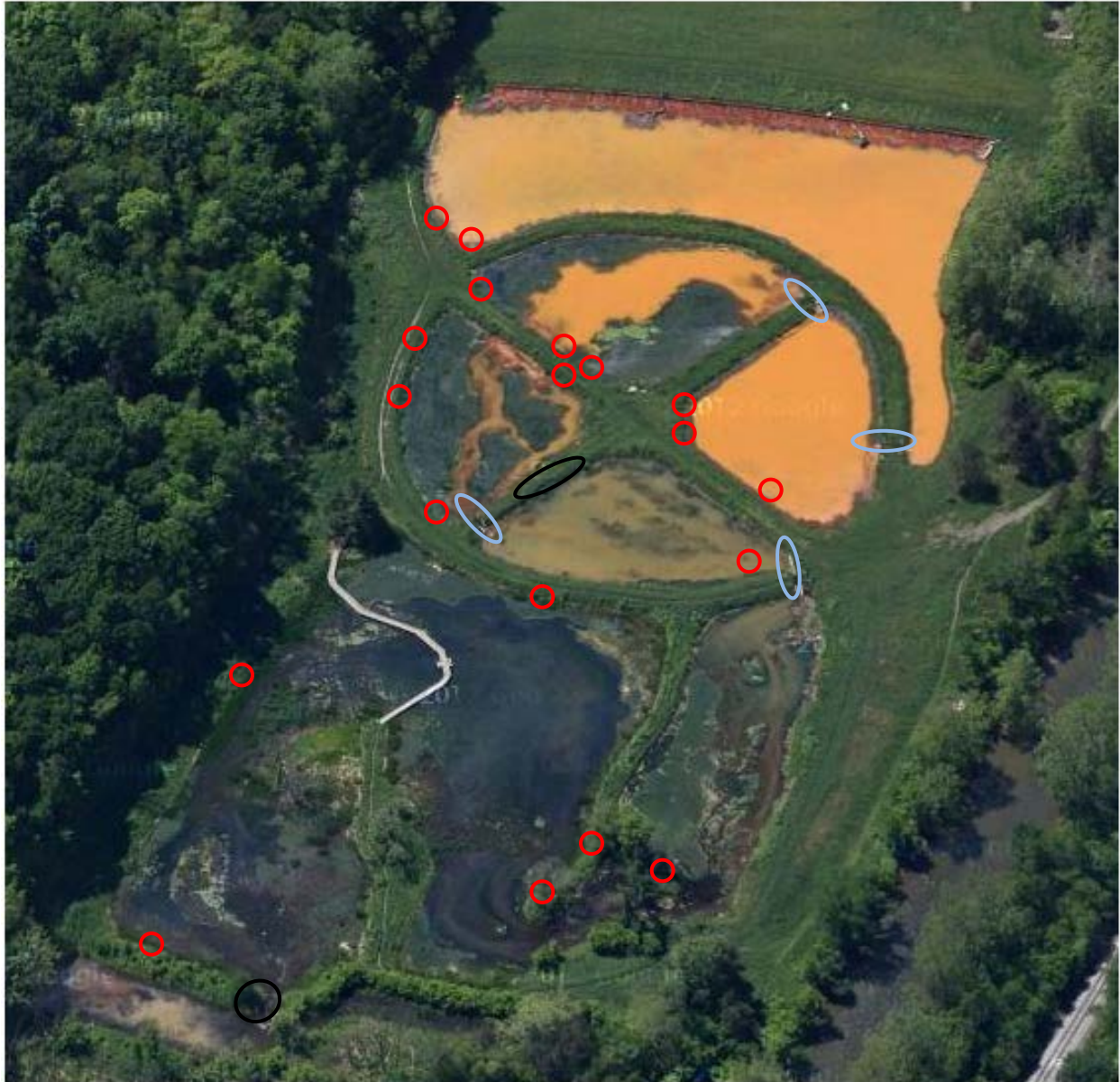
Figure 6. Problem areas at the Wingfield Pines site. Red circles indicate muskrat damage, blue circles indicate erosion around grates, and black circles berm slumpage or erosion.
