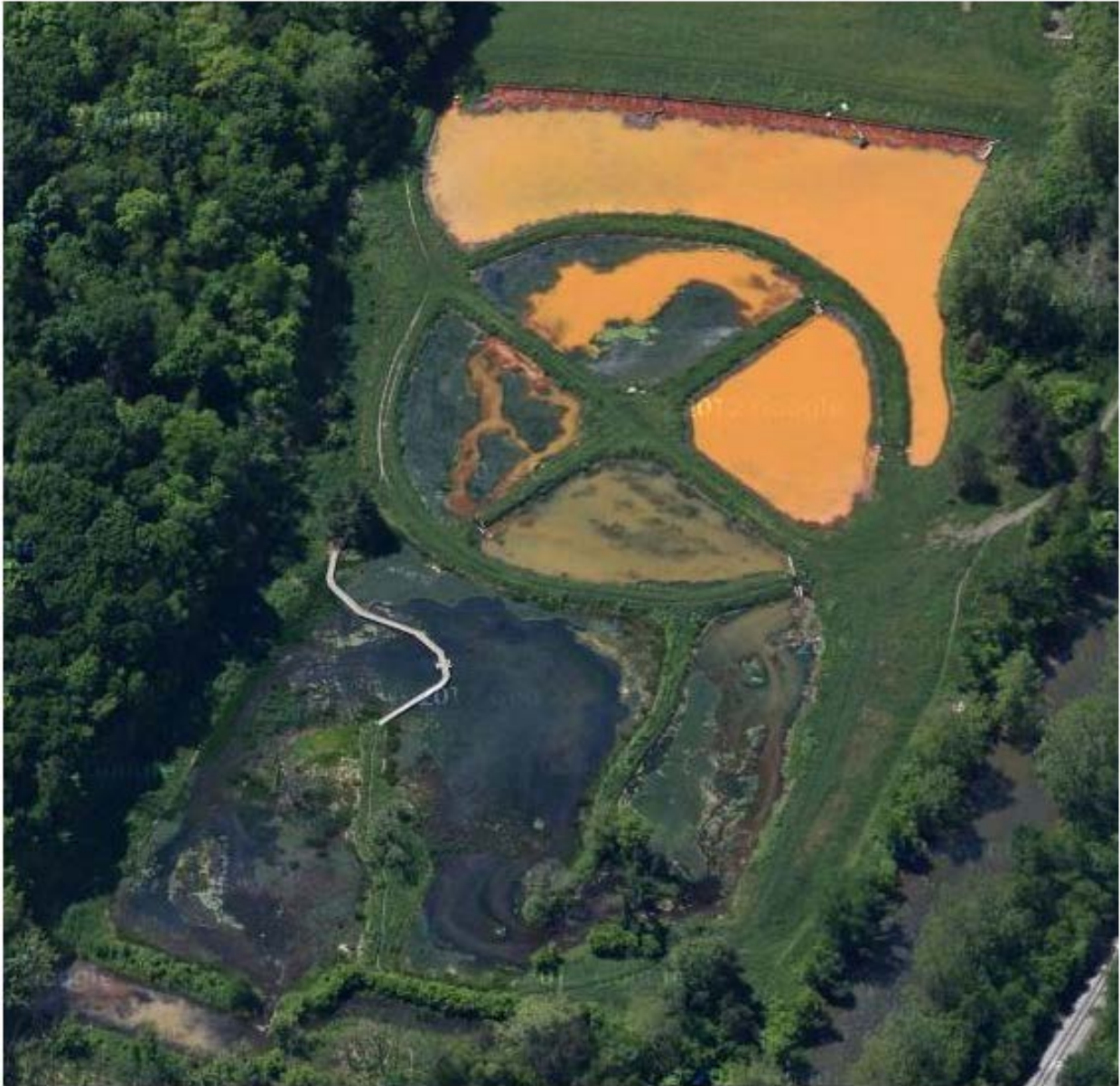
Figure 1. The Wingfield Pines passive treatment system on August 12, 2012. Water flow from the top of the photo through the ponds and into the wetland on the bottom of the photo. The growth in the ponds and the first wetland section is largely muskgrass, Chara spp. . The muskgrass is a very good filter and its effective removal of Fe solids is apparent by the lack of orange color in the wetland.
